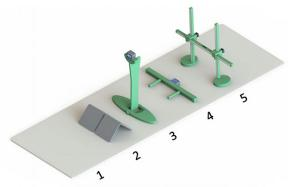
*Note.* Anatomical measurement instrument with equipment listed from left to right: 1 = non-slip mat; 2 = foot brackets; 3 = leg paddle with level box angle sensor; 4 = pelvic bridge with level box angle sensor; 5 = chest frame (Goldsmith & Goldsmith, 2013).
